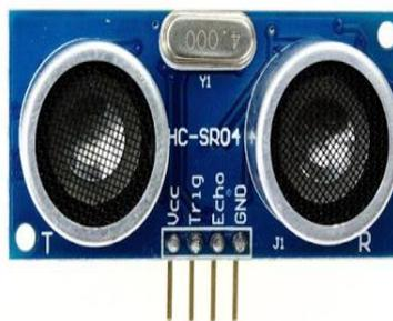
**Gambar 6.** Sensor Ultrasonik
