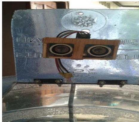
**Gambar 16.** Sensor Ultrasonik
