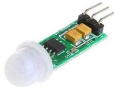
Gambar 8. Sensor PIR (*Passive Infra Red*)
