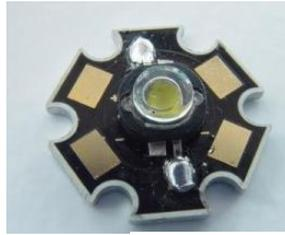
Gambar 11. *LED (Light Emitting Diode)*
