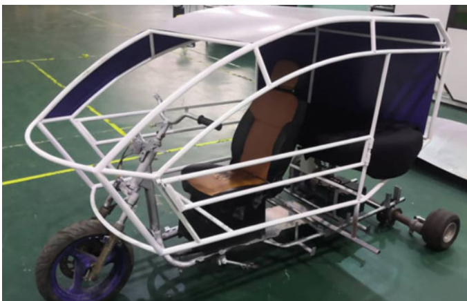
Fig. 4 Electric vehicle structure fabrication and configuration
