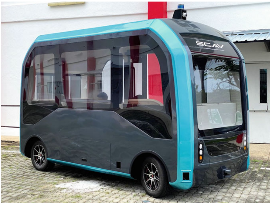
Fig. 1 Autonomous prototype of compact shuttle with camera and lidar sensor mounted on top
