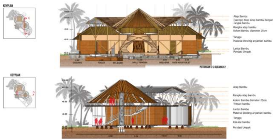
Figure 9. Building section Source : Researcher's analysis, 2022
