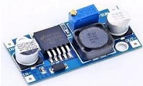
Gambar 6: DC Converter LM2596.
