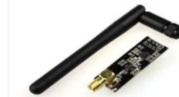
Gambar 4 Modul Transceiver nRF24101
