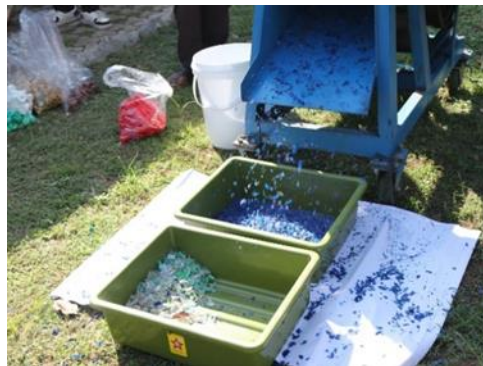
Picture 4. The Plastic Waste Shredding Process Workshop (Source: Private Documentation, 2024).
