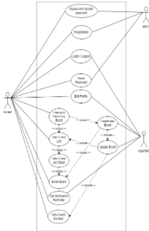
Figure 2. Use Case Diagram System Recommendation Event Platform
