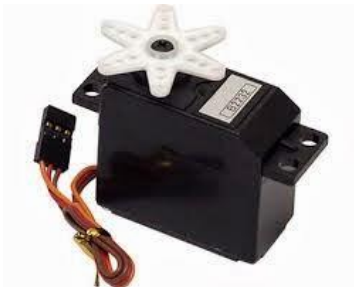
Gambar 2.7 Motor Servo (Sumber: Deby, 2017)
