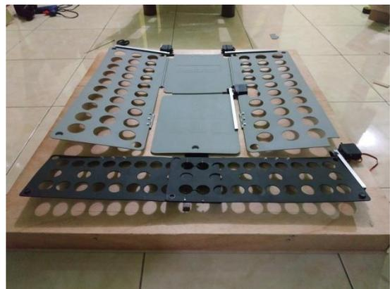
Gambar 11: Mekanik Alat Pelipat Baju Otomatis
