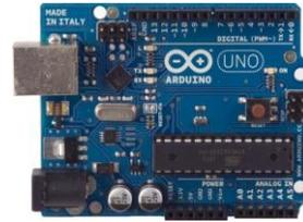
Gambar 1: Board Arduino
