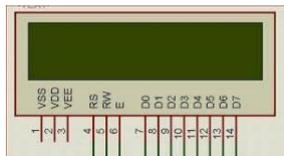
Gambar 3: LCD 2x16
