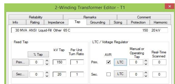
Gambar 4.3 Pengaturan Load Tap Changer (LTC) / Voltage Regulator
