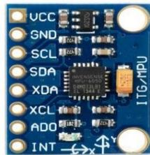
**Gambar 2.7** Sensor MPU
