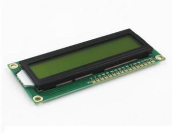
**Gambar 2.5** LCD 16 x 2
