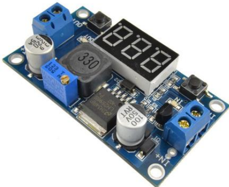
Gambar 2.9 Step Down Lm2596 (Sumber: Arduino-shop.cz )
