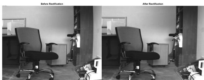
Fig. 6. Distorted images correction. (left) The image before correction. (right) The image after correction.
