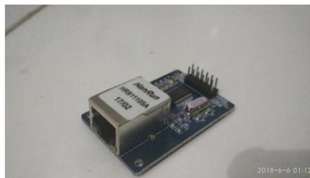
Gambar 1. Ethernet Module
