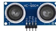
Gambar 2.2 Sensor Ultrasonik
