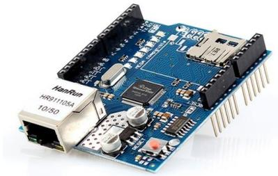
Gambar 2.2 Ethernet Shields
