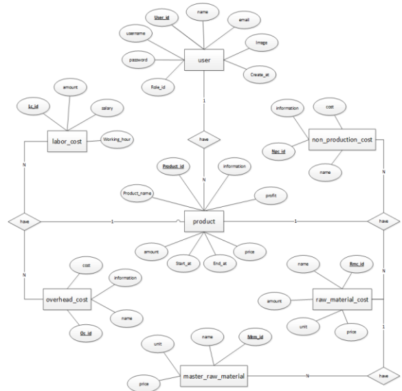
Gambar 6: Entity Relationship Diagram (ERD)
